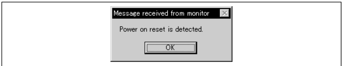
Figure 6.3 Power-on Reset Input Message Box
