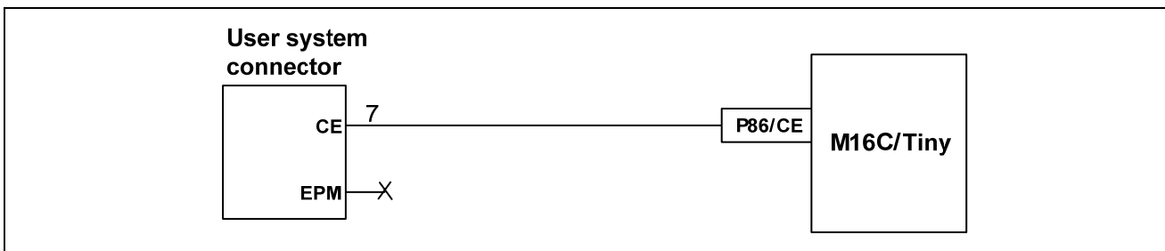
Figure 5.3 Connection of E8 Emulator and Pin P86
