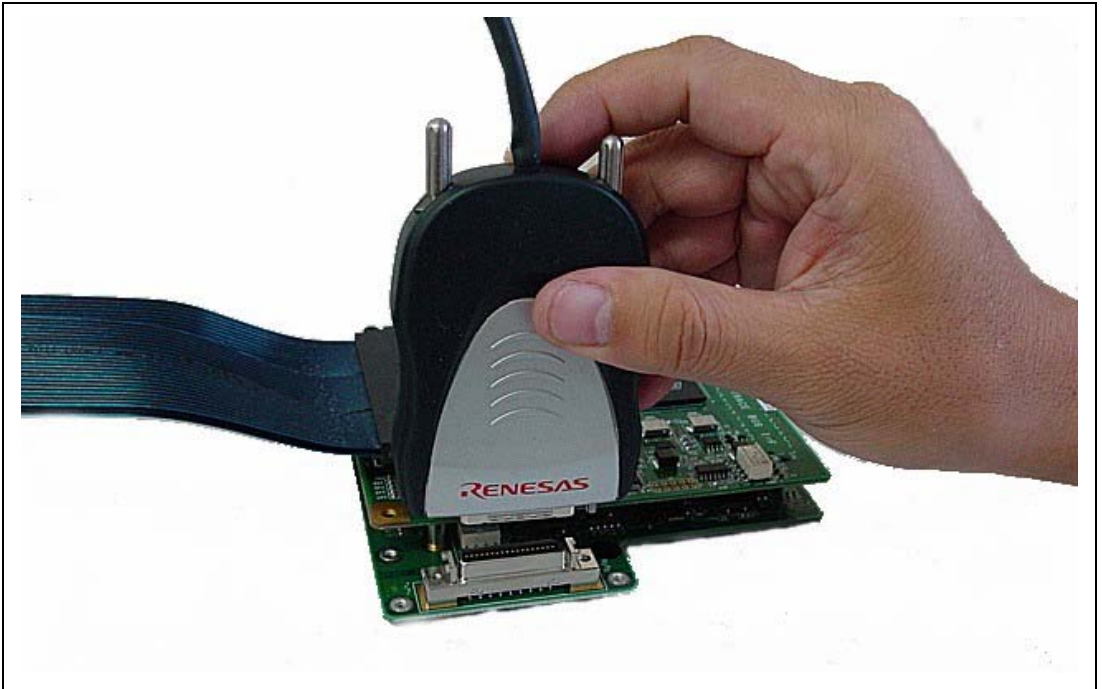
Figure 2.5 Connecting the H-UDI/AUD Probe to the EV-chip Unit
