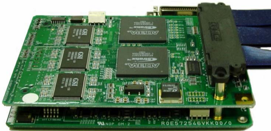
Figure 2.4 Connecting the Expansion AUD Trace Unit, EV-chip Unit, and Trace Cable
